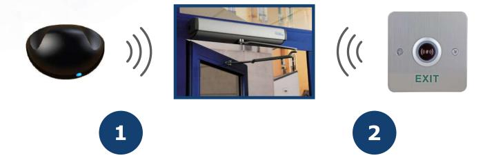
A microwave sensor detects a person approaching a DIGIWAY door, and triggers the door operation automatically.
